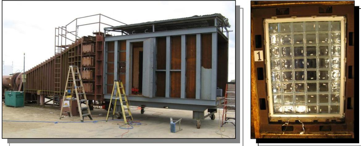
Six 4 feet by 5.33 feet panels were tested at the shock tube facility at BakerRisk. Utilizing sophisticated blast testing, data collection, data analysis and numerical modeling techniques, BakerRisk was able to produce a report delineating the Design Limit and Elastic Limit for panel sizes that would provide the ASTM "Minimal Hazard" or GSA "Performance Condition 2" levels of protection.
