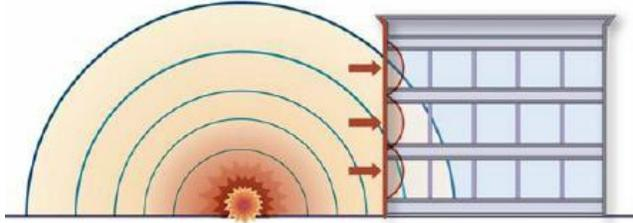
The actual effect of a blast is a function of its type, magnitude, duration and distance from where the blast took place. Standoff distance is a distance maintained between the building and the potential location of an explosive detonation, like a sidewalk or parking lot. Standoff distances will be longer where there is potential to detonate a larger explosive device, like one driven in a car, and shorter where the device could be carried.
