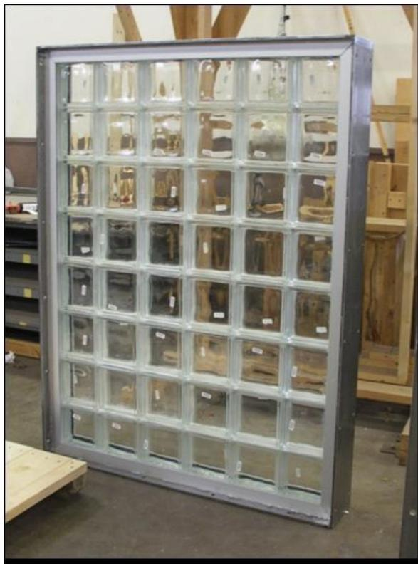
Alternatively, the blast resistant system could be installed utilizing the aluminum two-piece channel. This channel allows for the first piece of the frame to be attached to steel, masonry
